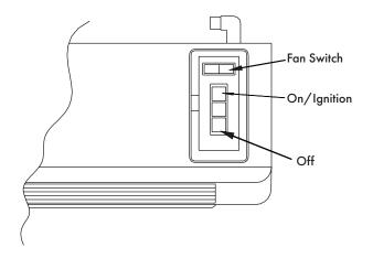
The ON/IGNITION/LOW button and the MEDIUM/HIGH button each have two operating positions, which provides three heat settings.
