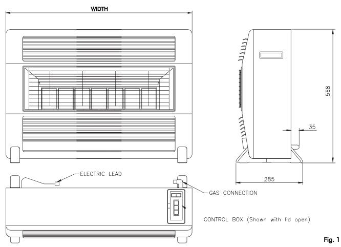
\*Electrical connection located 70mm in from Left Hand Side of Gas Space Heater
