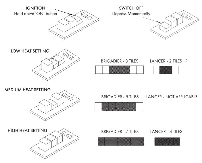
Low, medium and high settings can be obtained by setting the buttons set as shown in the diagrams above. If you depress the button firmly and it remains in the half way position, a second depression will return it to the fully up position.
